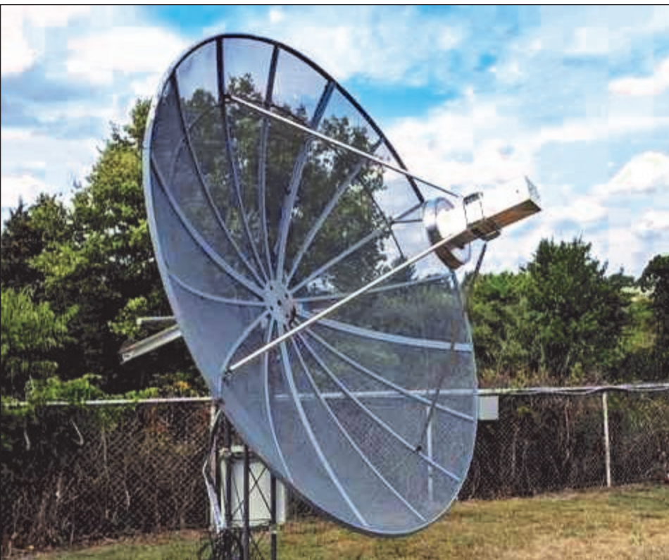
10' dish and feed at the DVRA club site with K1JT et al operating W2ZQ on 1296MHz
